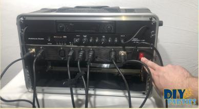
At this point, everything's plugged in, so go ahead and switch on your mains power supply, and the big red switch - and things should start to turn on! You'll see the devices in the rack light up, and the speakers & lights should boot up as well!
