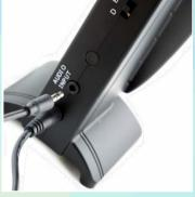
Connect the supplied 3.5mm (minijack) audio cable to your device, and to the audio input on the transmitter. For the pro one, you'll need to use the RCA adapter too as pictured.
