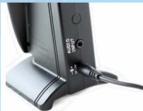
Start by connecting power (you can use the internal battery instead on the professional transmitter). Simply plug in the provided cable to the power port on the transmitter, with the other end plugging in to the venue's power supply.
