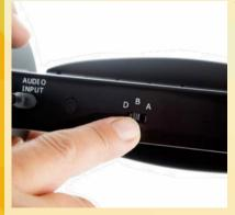
The last step is to select a channel using either the sliding switch on the basic, or button & screen on the pro transmitter.
